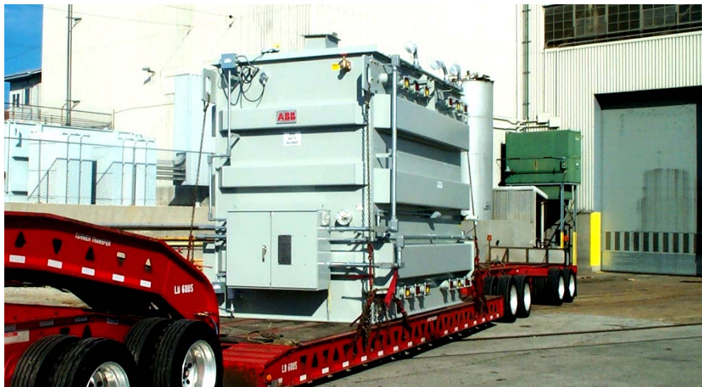
Figure 28: The EPRI/DHS Recovery Transformer will be quickly transportable to a substation for rapid installation and energization.
